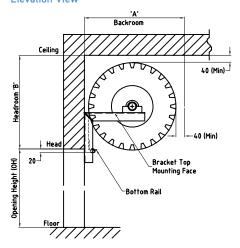
The structure to which the brackets and tracks are to be mounted must be of sufficient strength to accommodate the loads imposed by the roller door. The surface on which the brackets and tracks are mounted should be extended up above the lintel and be flush with or slightly behind the lintel.
